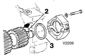
Set driving ball (76/2) into bore of interm. shaft.
