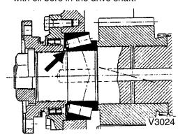
**3** Apply LOCTITE 243 to threads on input and output shafts.
