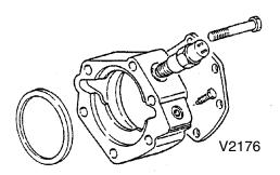
8 Remove the retaining ring (8/1) and speedometer gear (8/2) from the intermediate shaft. Pay attention to the driver ball.
