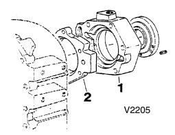
Mount bearing housing (70/1), with intermediate plate (2). Put driver ball (70/1) into dead end bore of drive shaft with grease
