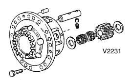
7 Separate rear axle output shaft (136/1) from ring gear (136/2) by removing retaining ring (136/3).
