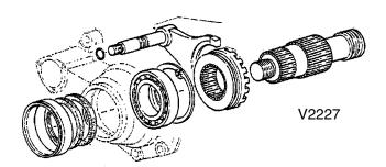
13 Install shifting fork (119/1) and shifting sleeve (119/2), into the housing with the shift dogs facing up.
