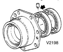
3 Press roller bearing (46/4) into the bearing carrier with support disk TS 213 W (47/1).
