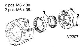
6 Mount rear bearing housing lid (73/1) (on bearing housing) with DIRKO sealant.
