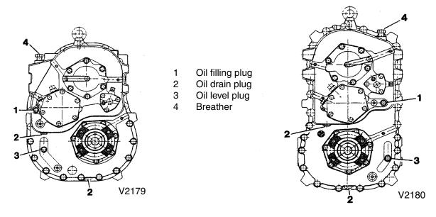
Drain oil by unscrewing both oil drain plugs (2)
