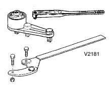
3 Pull-off flanges from the shafts with extractor A/VG 2000-05 (3/1).
